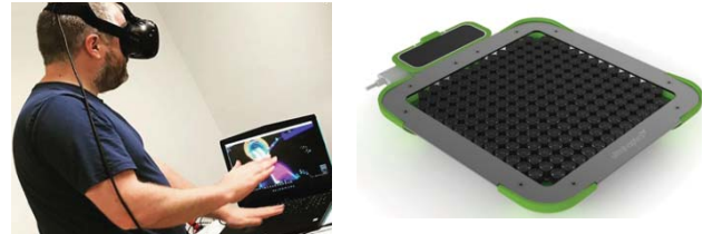
Figure 1: Photo of the demonstration setup, the UHDK5 device, and the LEAP motion controller.
